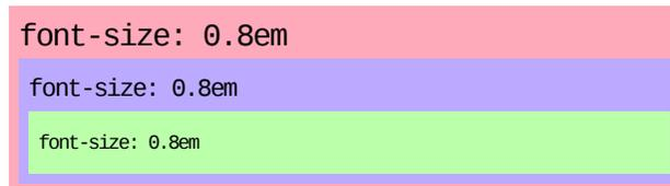
The diagram shows three nested rectangular boxes, each containing the text 'font-size: 0.8em'. The outermost box is pink, the middle box is purple, and the innermost box is green. This illustrates how the font size of the innermost box is calculated as 0.8 times the font size of its parent (the purple box), which is itself 0.8 times the font size of its parent (the pink box), demonstrating the compounding effect of relative units.
